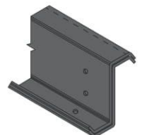
Nesting of Two Purlins
